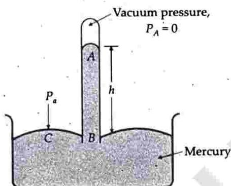
Fig. 10.11 Mercury barometer.
