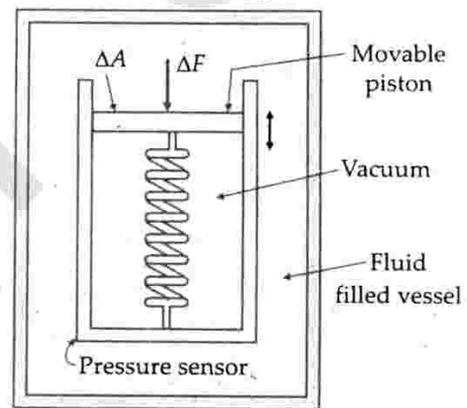
**Fig. 10.2** Measurement of fluid pressure.
