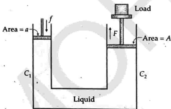
Fig. 10.5 Hydraulic lift.
