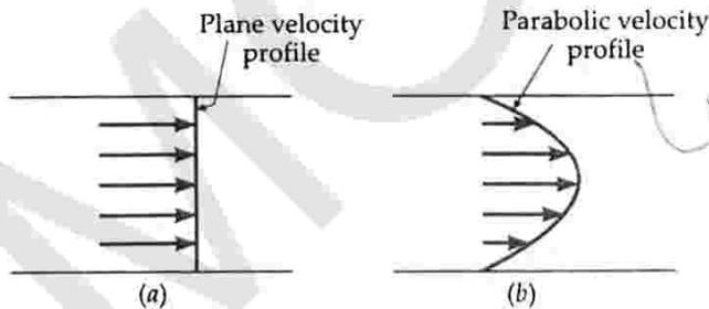
**Fig. 10.30** Flow of (a) Non-viscous (b) Viscous liquid through a pipe.
