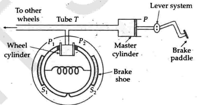
Fig. 10.6 Hydraulic brakes.
