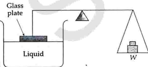
Fig. 10.52 Measurement of surface tension.
